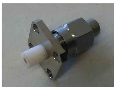
Figure 4. SMA connector with dummy load
