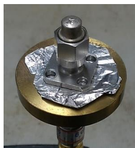
Figure 5. SMA connector insertion into the jig
