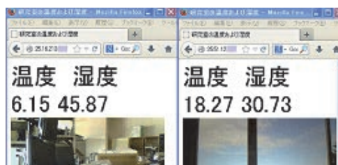
Figure 5 Details of camera image and temperature/humidity information provided via a Web browser
