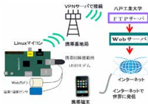
Figure 2 Configuration of a system using Web server that displays sensor information transferred via VPN to FTP server
