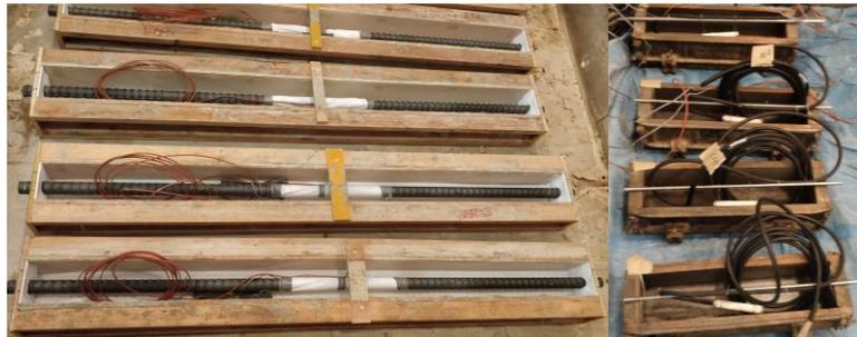
Figure 3.3. Uniaxial restrained and free shrinkage.
