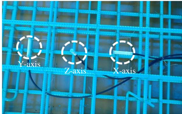
(a) Embedded strain gauge measuring point setting
