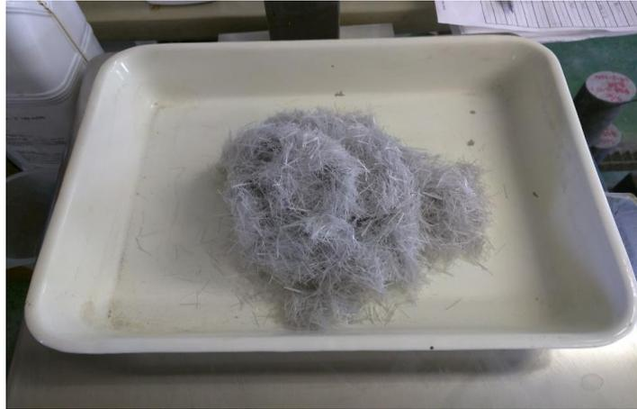
Figure 4.13. Polypropylene fiber.
