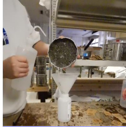
Fig. 4-6 Freeze-thaw scaling amount collection
