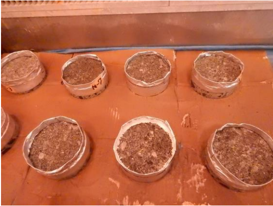
Fig. 4-5 Freeze-thaw state of the specimens in the freeze-thaw weather room (20th year)
