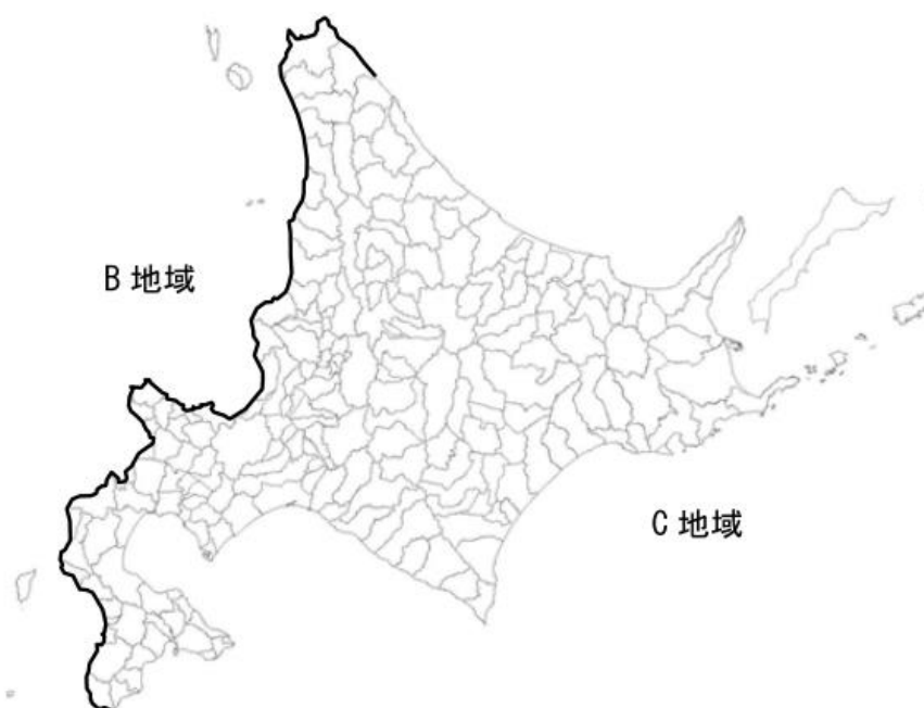
Fig. 5-1 Geographical distinction of the degree of influence of salt damage [120, 121] 2-29
