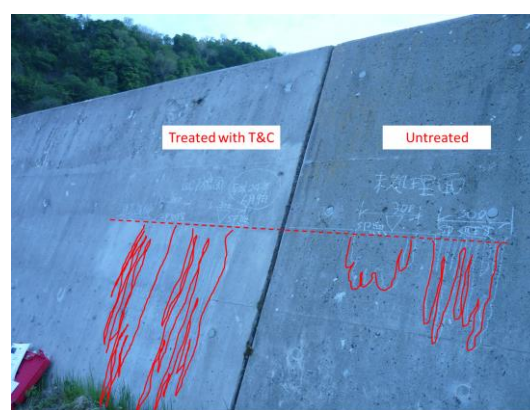
Fig. 4-2 On-site situation —The effect durability of surface water repellency (watering test)(12 th )
