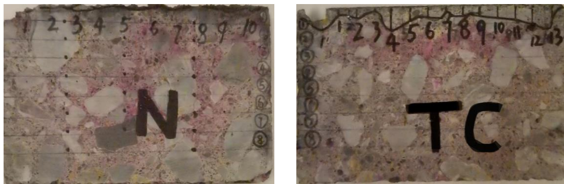
Fig. 4-9 Carbonization depth 20 th after construction (N: Untreated groups; TC: treated groups )
